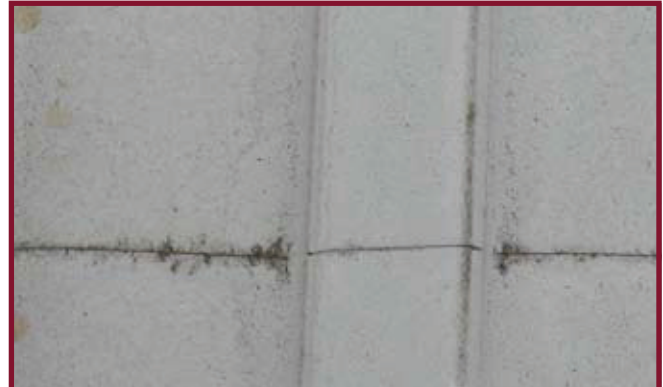
Manufacturer's defect (scribe) corrosion after 20 years
