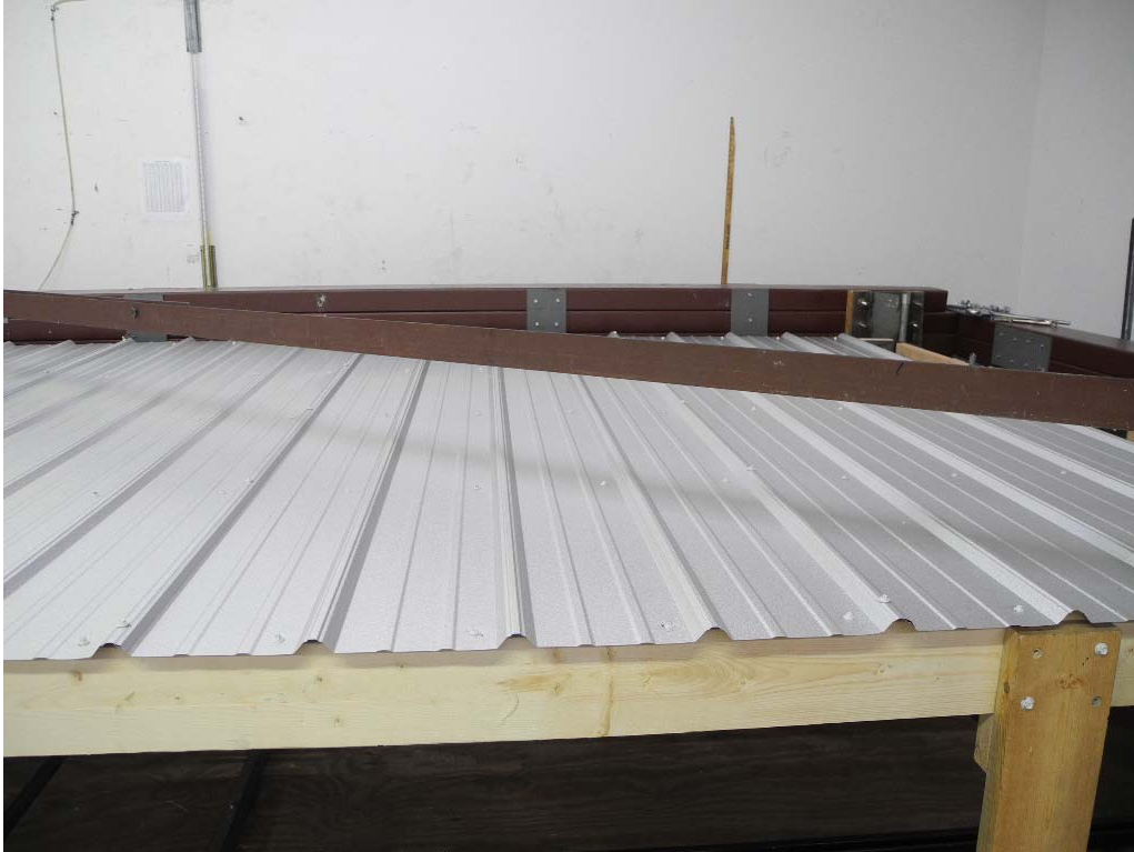
PHOTO 3 View of the panel fasteners at end and interior supports. (DSCN0011)
