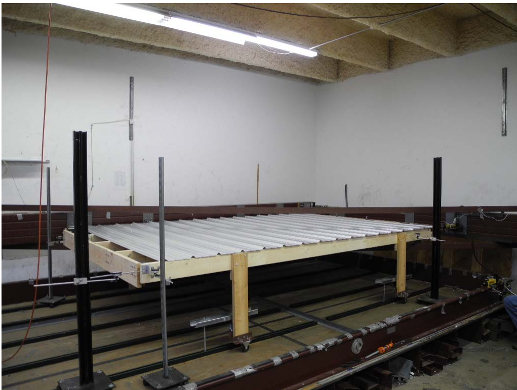
PHOTO 4 Overview of the diaphragm test setup of the Panel-Loc Plus at 2' 0" span. (DSCN0010)
