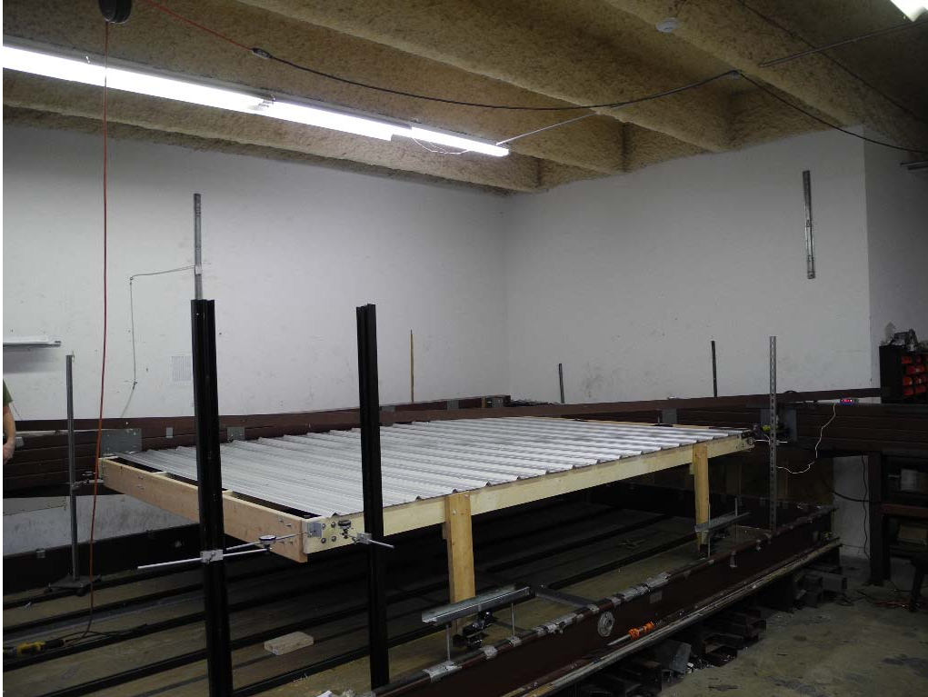
PHOTO 7 Overview of the diaphragm test setup of Panel-Loc Plus at 3' 0" span. (DSCN0027)
