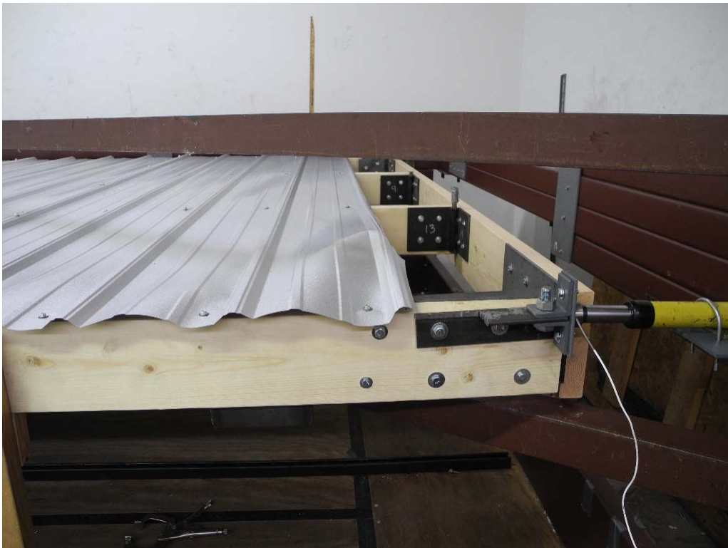
PHOTO 8 View of panel buckling near the loaded corner in Test #3. (DSCN0030)
