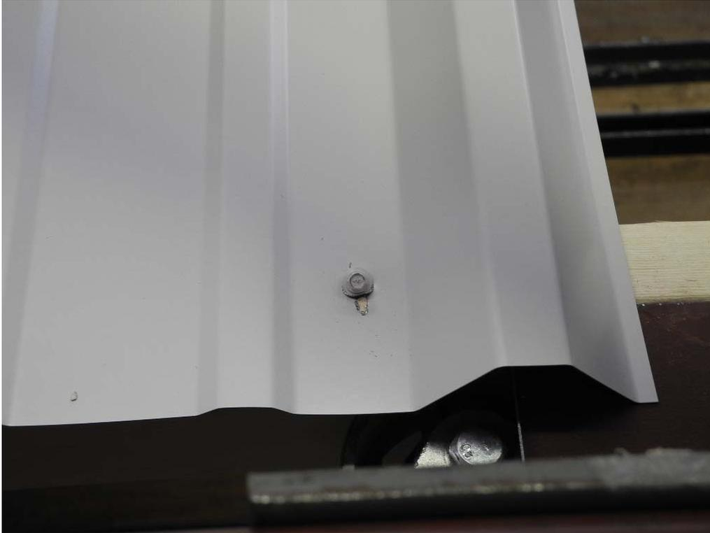
**PHOTO 5** View of panel slotting at fastener near the roller support in Test #1.
