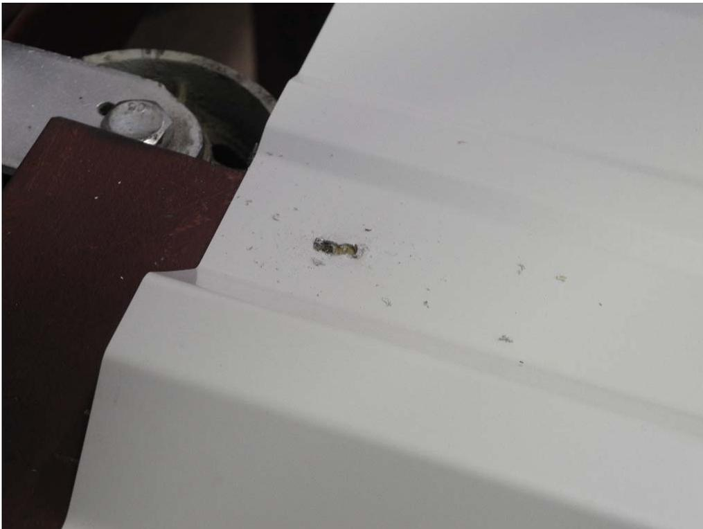
**PHOTO 6** View of panel slotting at fastener near the roller support in Test #2.
