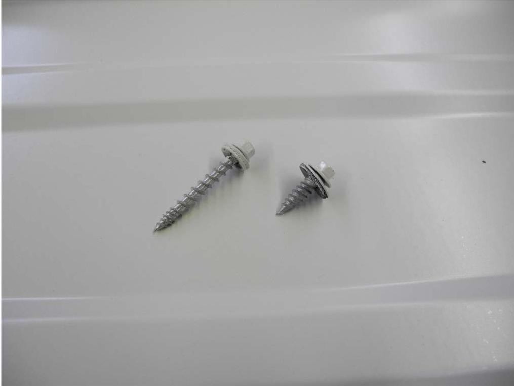
**PHOTO 1** View of the structural and sidelap fasteners.
