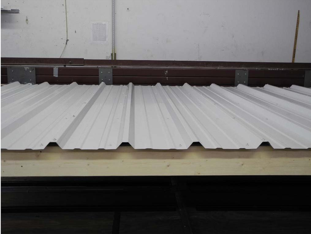
**PHOTO 3** View of the fasteners at end and interior supports.
