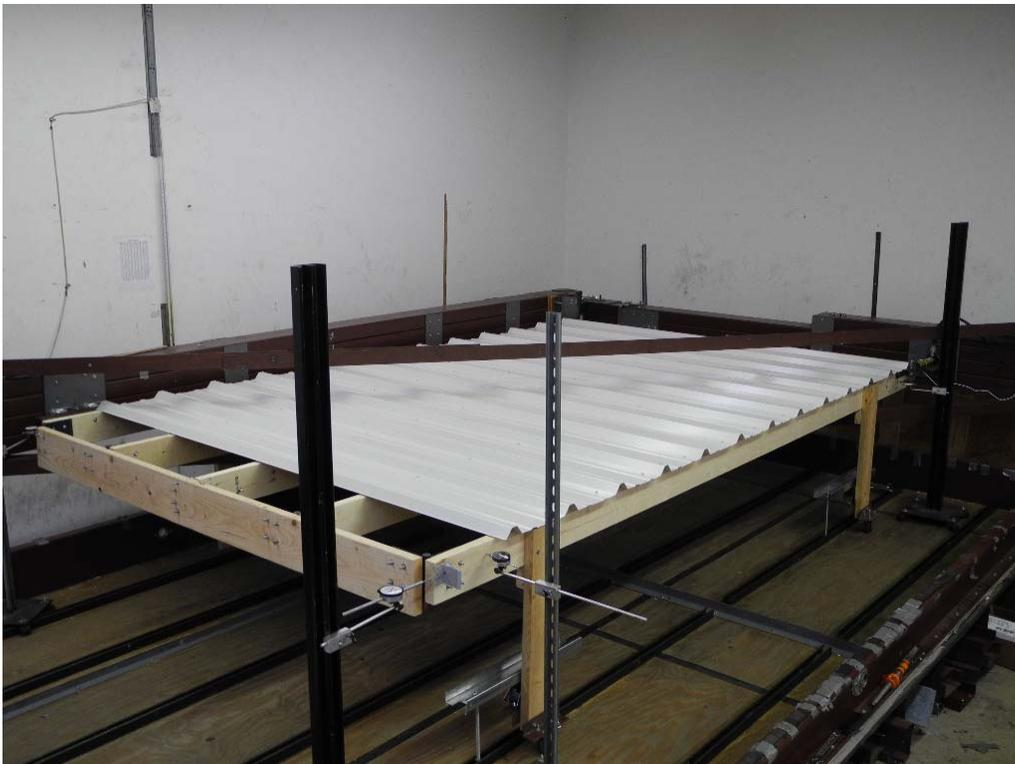
**PHOTO 4** Overview of the diaphragm test setup of the R-Loc panels.
