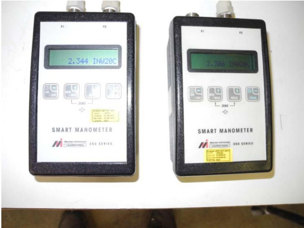
**PHOTO 5** View of flow measurements at differential pressure of 12.0 psf (equivalent to 2.306" of water). (DSCN3927)
