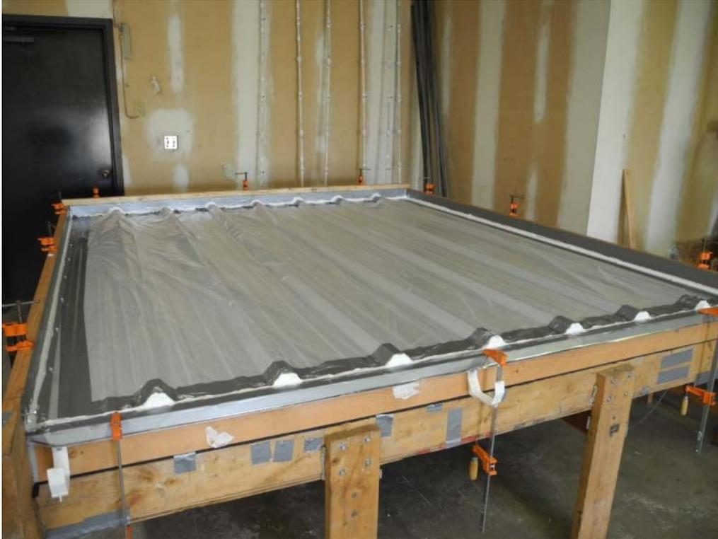
**PHOTO 3** View of test setup. The panel sidelaps and fasteners were temporarily sealed for extraneous leakage measurement of the test chamber. (DSCN3924)
