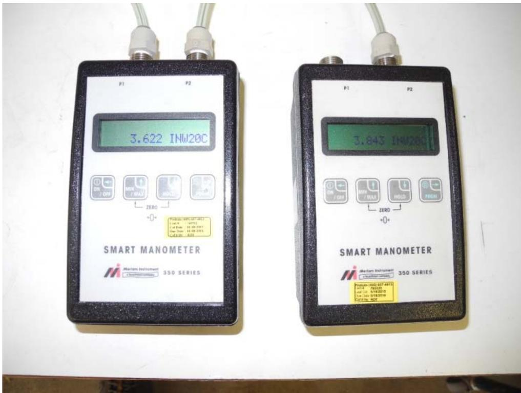
**PHOTO 6** View of flow measurements at differential pressure of 20.0 psf (equivalent to 3.843" of water). (DSCN3925)
