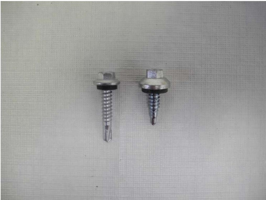
**PHOTO 2** View of panel and sidelap fasteners.
